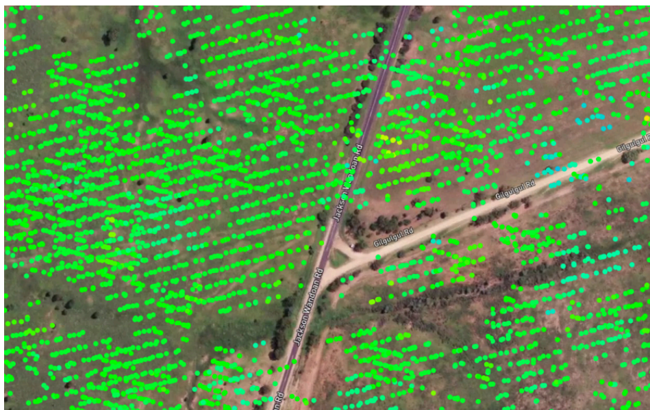
Figure 3. Example Persistent Scatterer Interferometry point coverage across Jackson Wandoan - Gilgulgul road intersection
