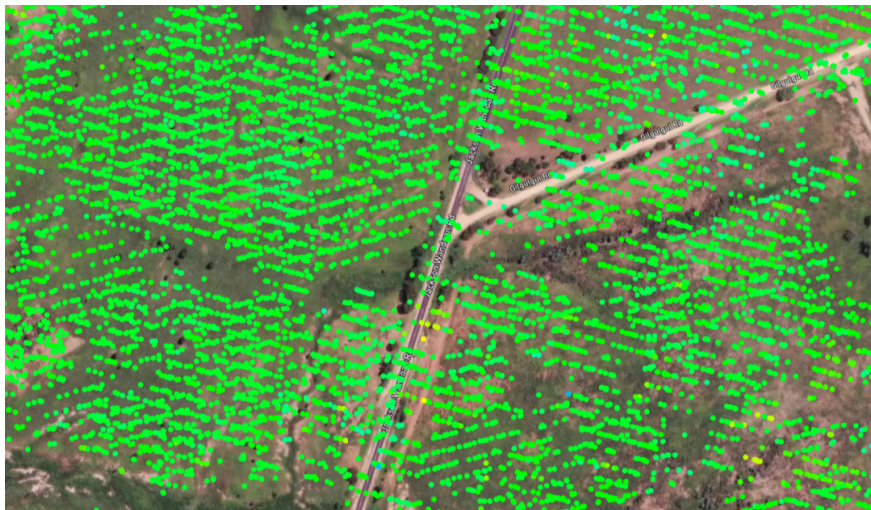
Figure 3. Example Persistent Scatterer Interferometry point coverage across Jackson Wandoan - Gilgulgul road intersection
