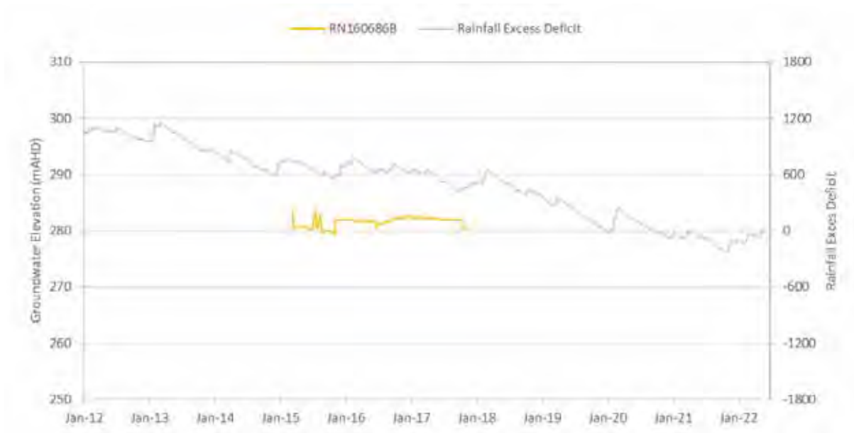
Figure 7.29 Groundwater Elevation Hydrograph – Evergreen Formation
