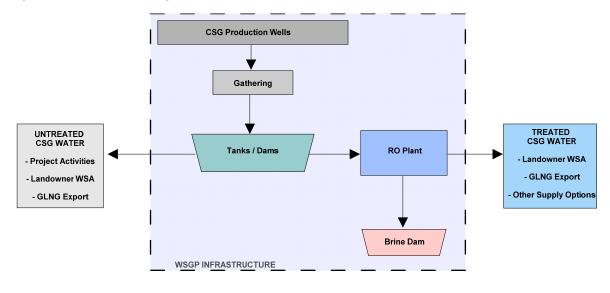
Figure 1.1 Water Management Infrastructure Schematic for the WSGP
